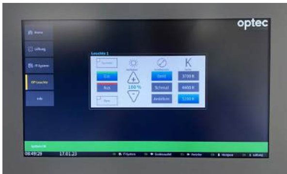
The CP915 control and operator units control all systems in the operating theatre and provide staff in the operating theatre with clear information on any disturbances that occur.
