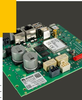
The ICC1314 charge controller is the central element of a charging system and is designed for use with Bender IPM1xxx Power Modules.
